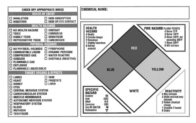
FIG. 11-2 Hazard codes used to label chemicals. (From Lab Safety Supply, Inc. Janesville, Wisc.)
