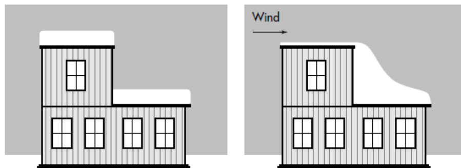
FIG. 5-5 Typical distributions of snow on roofs with different wind speeds. A , In calm conditions snow forms a uniform layer. B , If wind blows, the snow will drift. (Modified from O'Rourke MJ: Snow load on buildings, Am Sci 85:64-70, 1997.)
